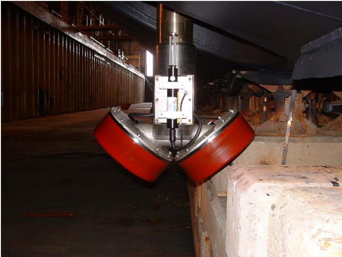
Figure 7 Sonar Head installation example: Retractable dual head
